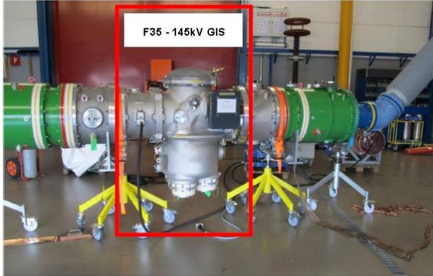
Figure 4. F35 145kV GIS - Dielectric test.
