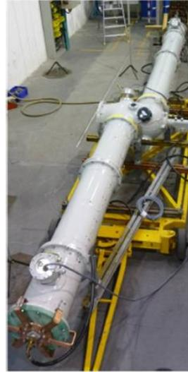
Figure 5. 420kV GIL temperature rise test.
