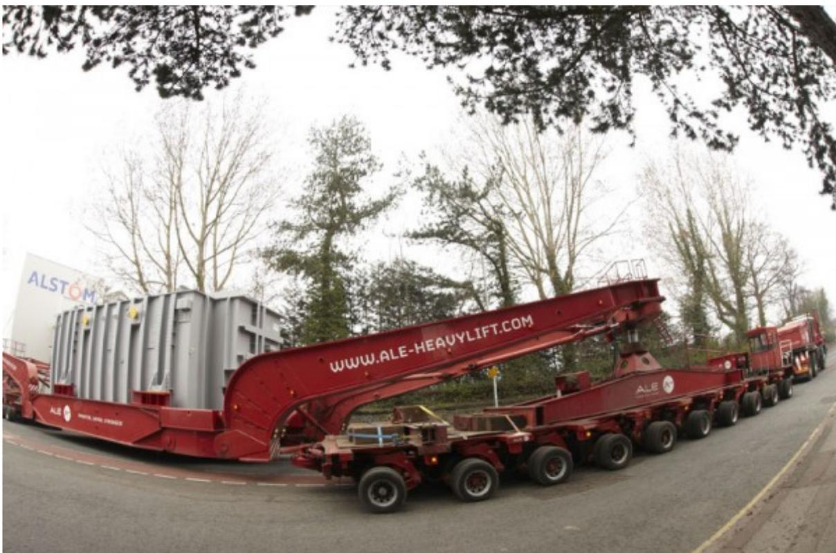
The size and weight of the 800 kV converter transformer is limited by shipping constraints
